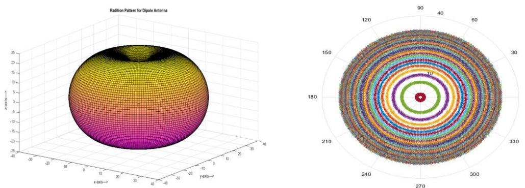
**Fig. 1:** 3D Radiation Pattern of Half Wave Dipole Antenna. **Fig. 2:**Power Distribution of the Omnidirectional Antenna in Horizontal Plane.
