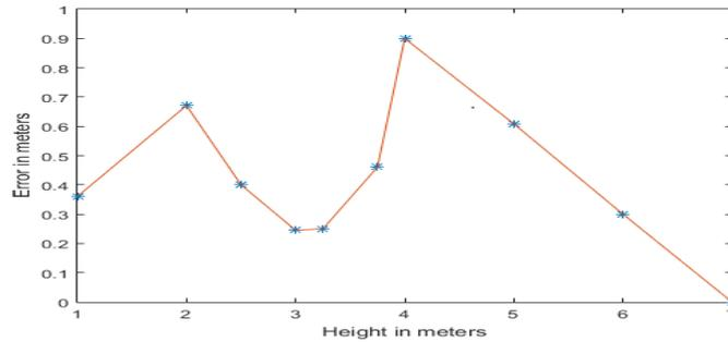
Fig. 4: Predicted location errorVsheight of the target nodes
